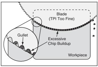
Figure 18. TPI too fine for workpiece.
